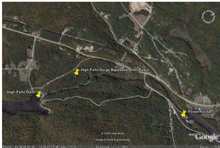
Map 1. Saranac river flowing from left to right through the High Falls Reservoir, High Falls Dam where water is removed, High Falls Gorge bypassed reach, and then past the powerhouse where water is returned to the river.
