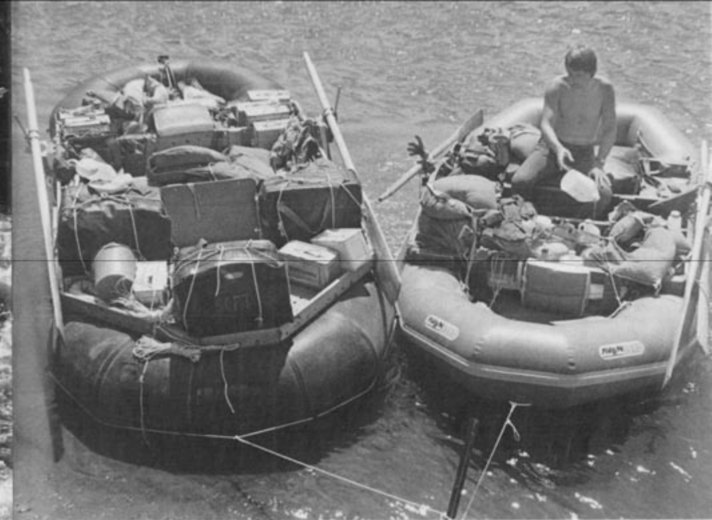
Elaborate frames not only greatly increase a raft's gear-carrying capacity, they also stiffen and stabilize the boat, rendering it snug, ship-like, and hard to wrap. Photo by Mike Gill.
