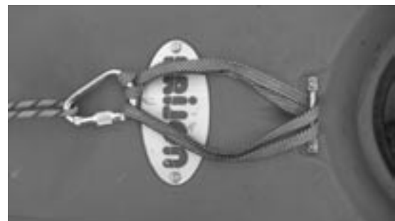
Above: Spectra climbing runner, grith hitched to wide end of a locking carabiner. To attach to a boat, feed the end of the runner through the bar or grab loop (you can add an extra wrap on a bar to cut down on the slide-around factor), then clip the end back into the carabiner, and close the lock. The girth hitch keeps the system clean and easy to use, especially when you are using the same setup for several boats in a row. The girth hitch does make the sling weaker, but it should still be much stronger than your rope.
