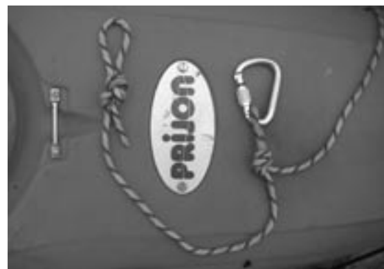
Below: The overclip. Tie an overhand loop on a bight about two feet from the end of your throwline. Run the end of the line through the bar or grab loop (an extra wrap on the bar cuts down on the slide-around factor), then clip the loops together, and close the lock.
