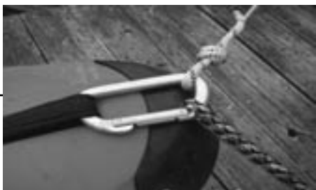
Three-way death load. Do not do this, even with a locking carabiner.
