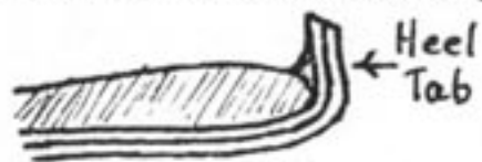
Fig. 3. Stick glue-coated sole pieces together as far as heel tab, bend top layer of tab up, then bend up bottom layer and stick them together.
