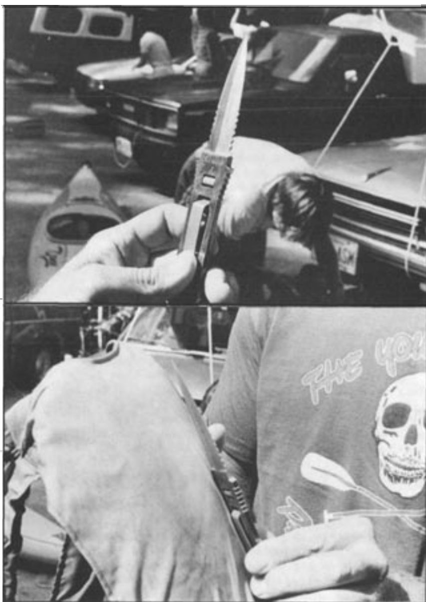
The two photos illustrate the flaw in the old "Clip Lock" design. In the top photo, the formerly exposed spring is evident. At the bottom, when the spring is compressed against a PFD, the blade's locking mechanism is released.
